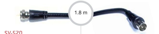
SV-570 Male F Male TV aerial/video TV aerial, video connection, etc. with coaxial RG-59U cable for radiofrequency signal and low power video connection Length 1.8 m
